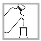
**8.** If the sample volume is less than 100 mL, dilute to approximately 100 mL with deionized water.
